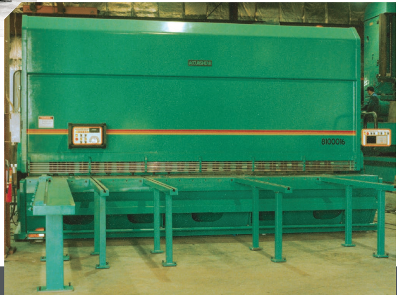
1" Capacity x 16' Accurshear
