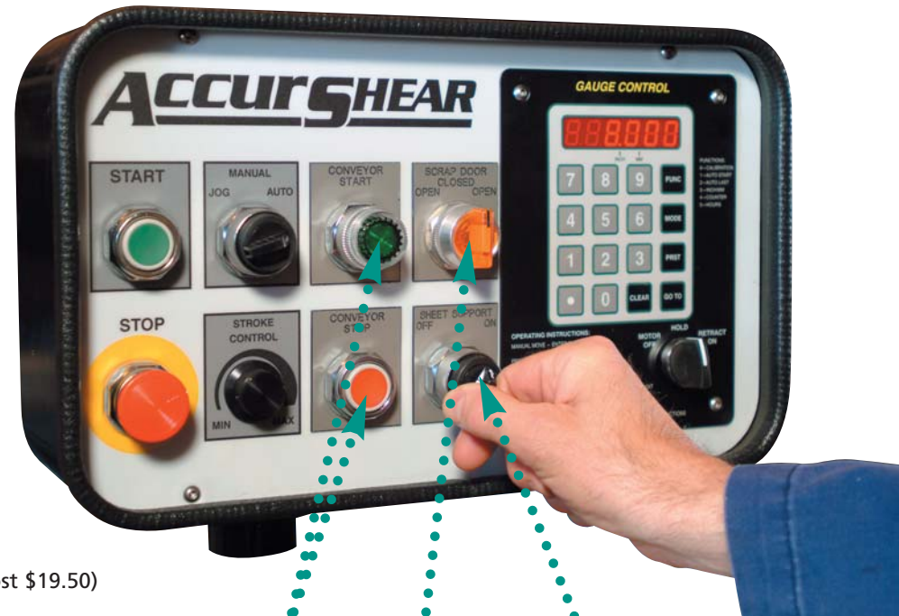
Conveyor stop/start Scrap door open/close Sheet support on/off
